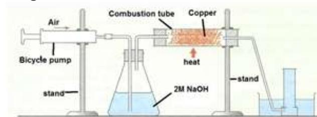
When air is passed through a solution of sodium hydroxide, carbon dioxide from the air dissolves in the alkali which removes carbon dioxide from the air.
