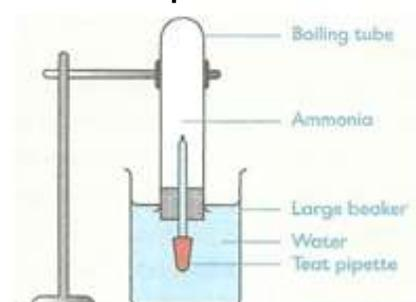
When a drop of water is released into the boiling tube containing ammonia, the water dissolves most of the ammonia gas, thus leaving a partial vacuum. This lowers the pressure inside the boiling tube. The rubber remains pressed inside because of atmospheric pressure.
