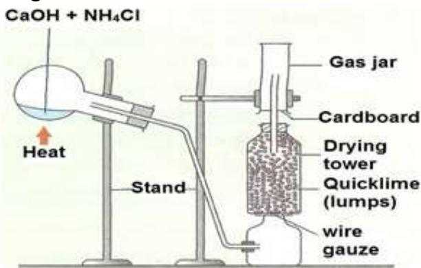
Calcium hydroxide reacts with ammonium chloride to produce ammonia gas, calcium chloride and water
