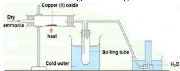
When ammonia gas is passed over heated copper (II) oxide, the gas is oxidized to nitrogen while the copper (II) oxide is reduced to copper.
