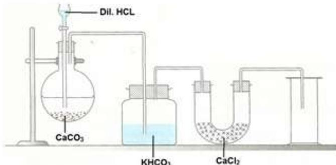
Dilute hydrochloric acid reacts with marble chips to give calcium chloride, water and carbon dioxide.
