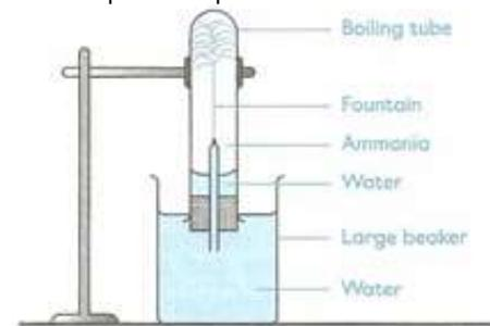
When the test is removed, the water in the beaker rushes into the boiling tube, thus dissolving the remaining ammonia gas. The water forms a fountain, thus the name of the experiment.
